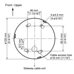
Locally procure four camera-mounting screws suitable for the installation surface and structure of the wall/ceiling or junction box. There are four 4.5 mm {3/16"} diameter screw holes and a guide hole on the camera panel.
